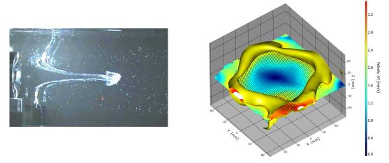
Visualization of the transient acoustic streaming jet generated with a transducer (left picture). Mean flow is obtained experimentally with reconstructed eulerian field from 3D particle tracking in an acoustic streaming configuration where the acoustic beam is oriented towards the wall of a cubic cavity with a 45° angle, resulting in several reflexions on consecutive walls (right picture).
